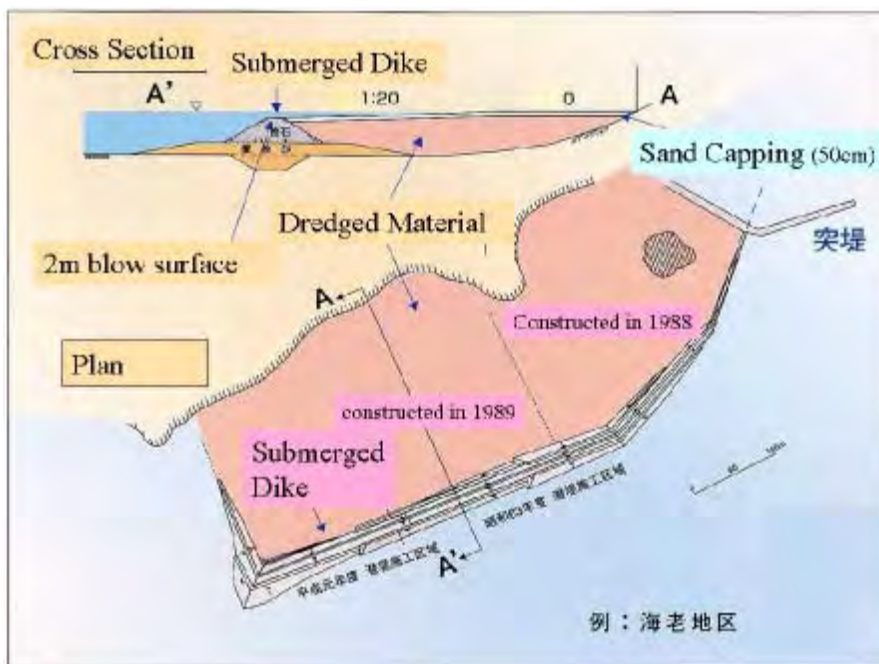
Figure 4-9 Mud flat habitat creation with underwater bund
