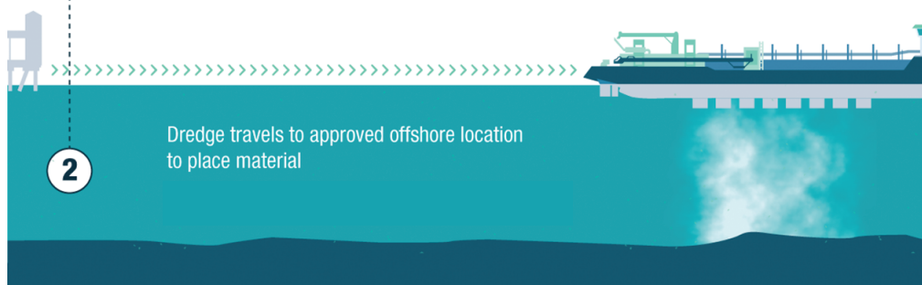
Figure 5.2 Trailing Suction Hopper Dredger placing material
