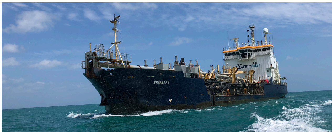
NQBP has used the TSHD (Trailing Suction Hopper Dredger) Brisbane for maintenance dredging in the past.
