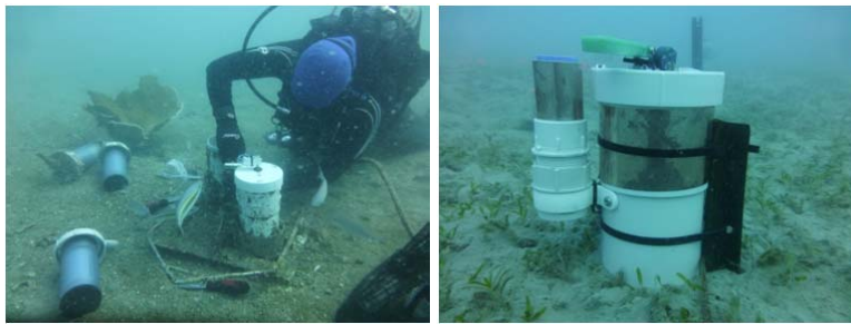
Figure 5. PAR & temperature loggers deployed at Abbot Point
