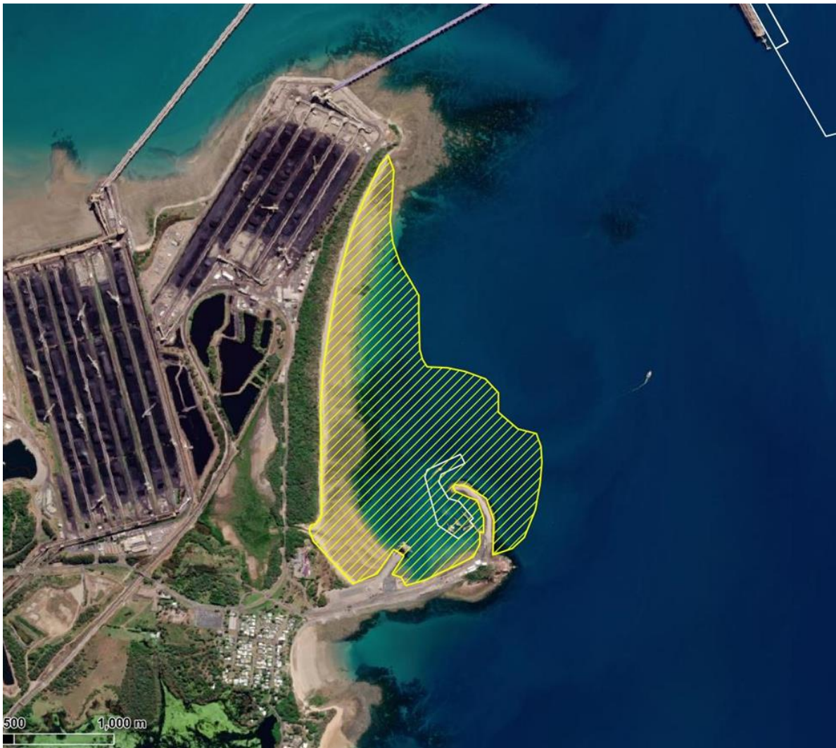
Figure 11: Zone of influence for dredging 60,000 m 3 from HTTH using a TSHD, based on 95 th percentile SSC being increased by more than 10mg/l as a result of dredging
