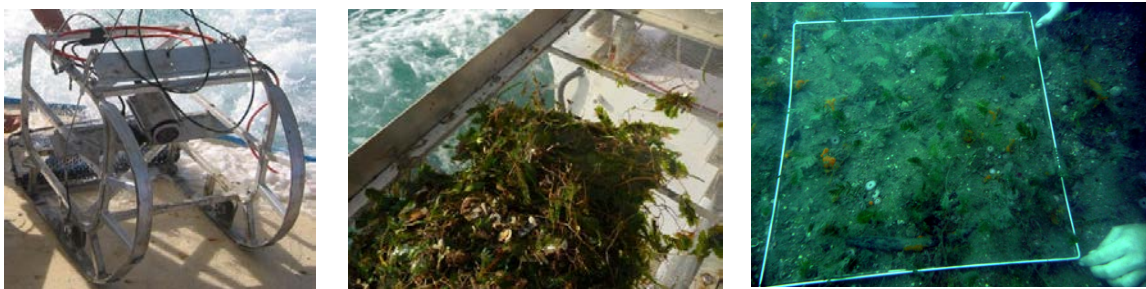
Figure 6. Sites were assessed by sled tows with digital camera free-divers to measure seagrass biomass and species composition.
