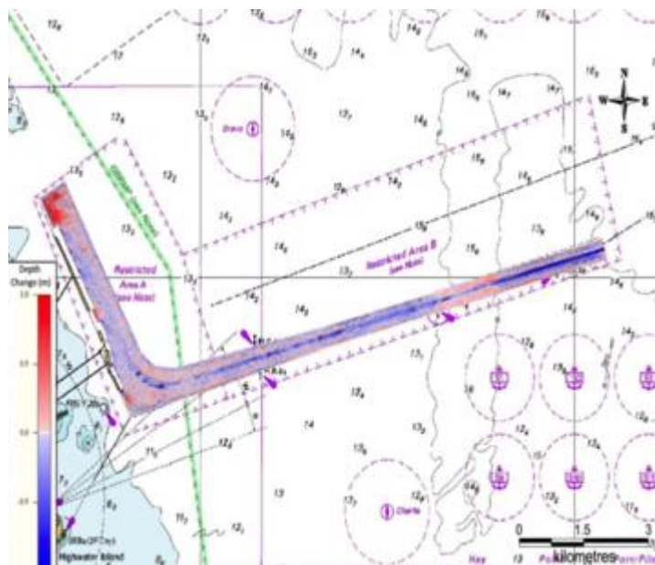
Figure 10: Difference in bathymetry (February 2007 to October 2015) red represents areas of accretion and blue areas of erosion
