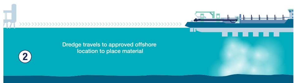
Trailing Suction Hopper Dredger placing material
