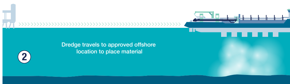
Trailing Suction Hopper Dredger placing material
