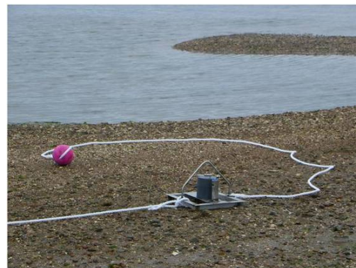
Deployed PAR logger in cradle on intertidal seagrass meadow
