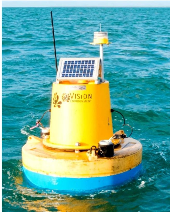
Figure 2 Dual surface telemetered physicochemistry monitoring station.
