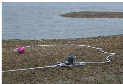
Deployed PAR logger in cradle on intertidal seagrass meadow
