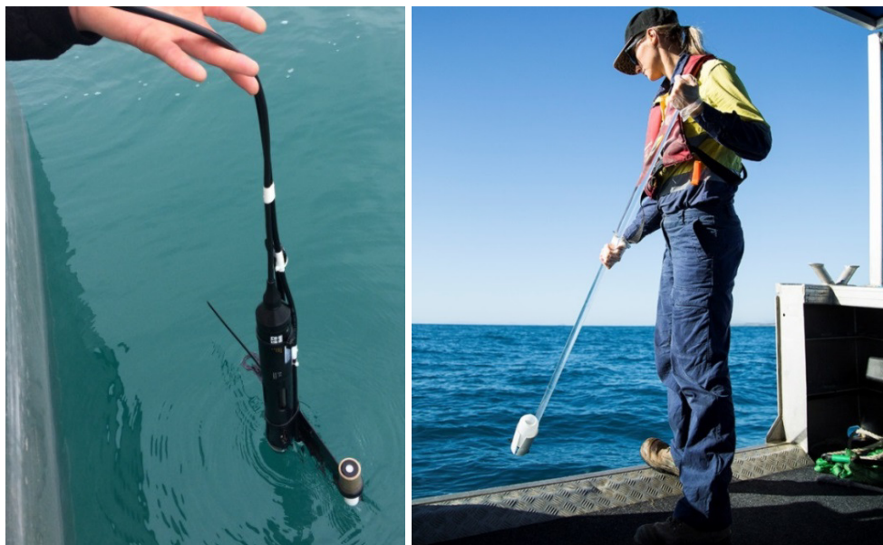
Figure 6 a) Depth profiling using the YSI ProDSS and the LI-COR LI192SA Underwater Quantum Sensor; and b) Collection of water samples for analysis using an acid-washed Nalgene bottle in a perspex pole sampler.
