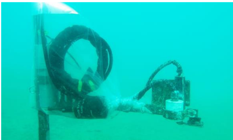
Figure 5 ALTUS altimeters deployed adjacent to continuous physicochemistry and BPAR logger frames.
