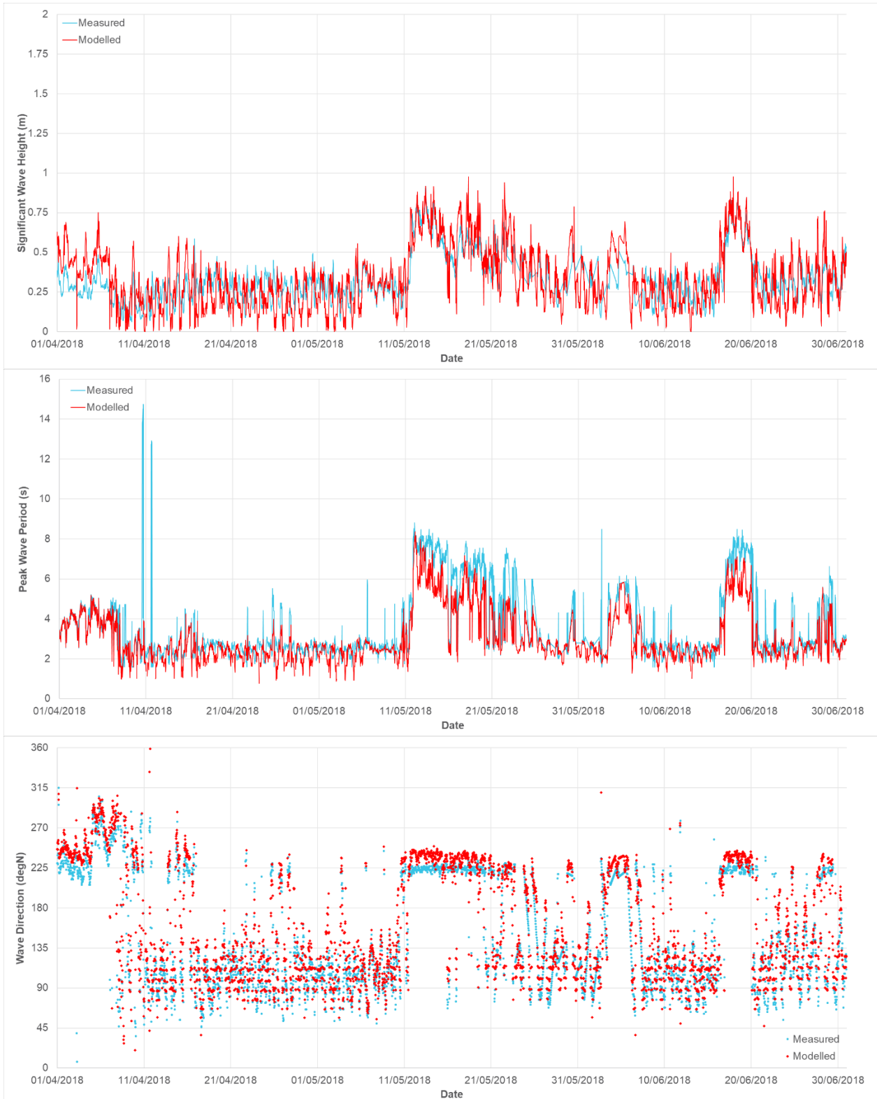
Figure 19. Comparison between measured and modelled wave conditions at the Albatross Bay WRB during the validation period.
