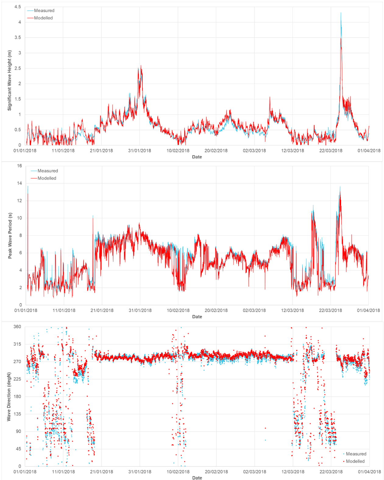
Figure 18. Comparison between measured and modelled wave conditions at the Albatross Bay WRB during the calibration period.
