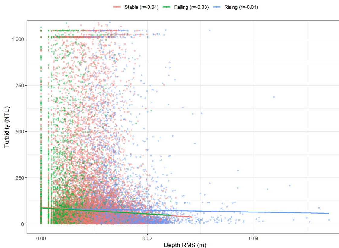
Figure 3-27 Relationship between turbidity (NTU) and RMS depth at Leithen Point (WP_AMB4) for the 2024–2025 reporting period. Scatter points are coloured by tidal stage, with linear regression lines and correlation coefficients ( r ) shown for each condition. Correlations are weak and negative, indicating limited coupling between near-bed wave motion and turbidity at this site.
