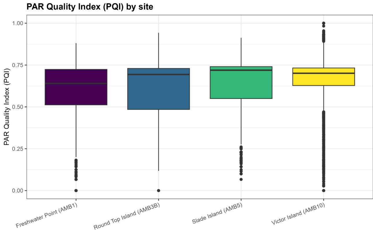
Figure 3—35 Boxplots showing the distribution of Par Quality Index (PQI) across the Mackay and Hay Point monitoring sites. PQI represents the proportion of benthic irradiance contributed by blue–green wavelengths (440–570 nm). Higher PQI values correspond to clearer optical conditions and greater availability of photosynthetically usable radiation (PUR). PQI was lowest at Freshwater Point and highest at Round Top Island and Victor Island.
