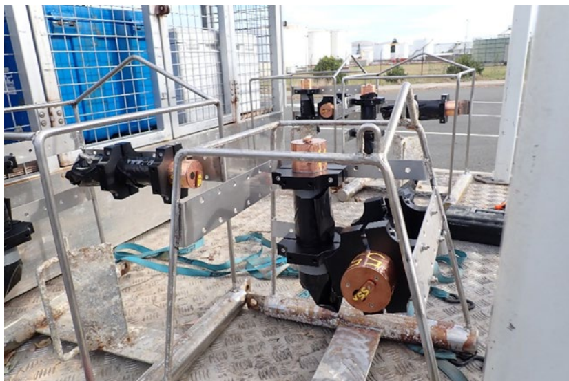
Figure 2—2 Water quality loggers attached to instrument frames ready for seafloor deployment. The horizontally oriented logger is an NTU-LPT turbidity logger; the vertically oriented logger is an MS9-LPT multispectral light logger (In-situ Marine Optics).
