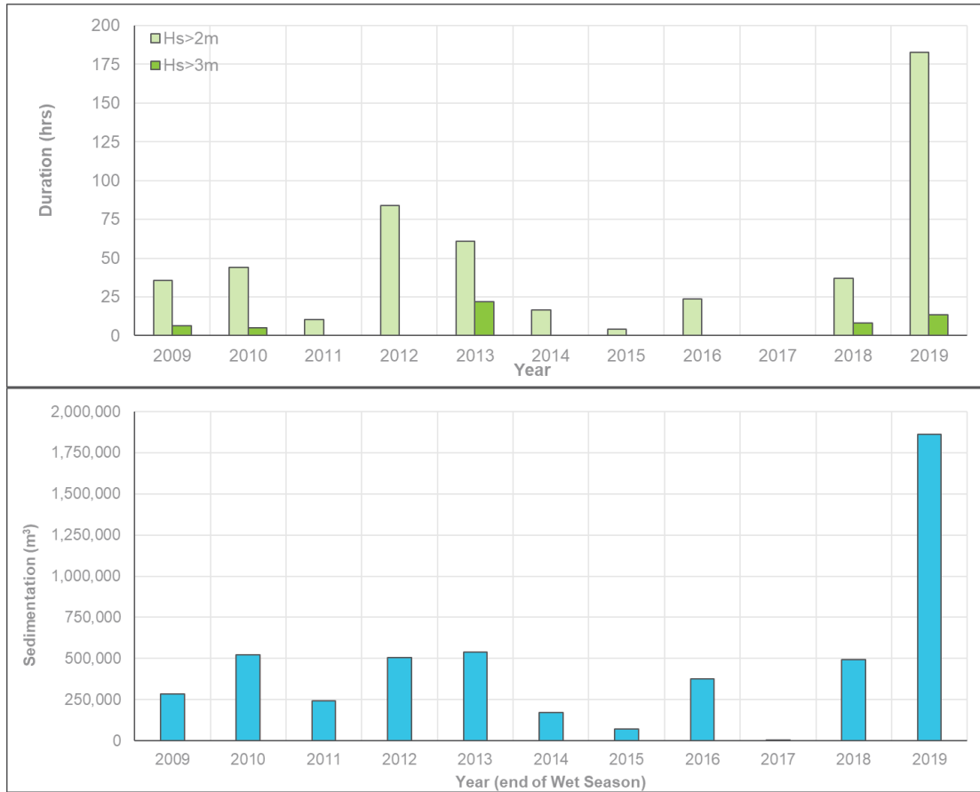
Figure 13. Total annual sedimentation in the South Channel (bottom) along with the hours that wave heights were exceeded each year at the Albatross Bay WRB (top).
