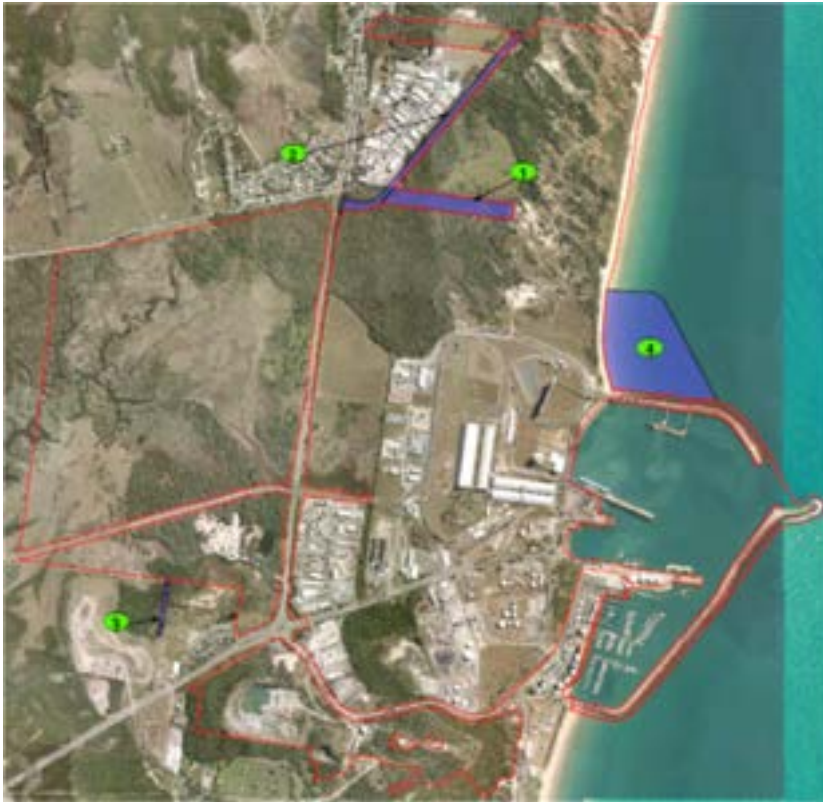
Figure 4-2 Port of Mackay Land Use Plan, Proposed Future Strategic Port Land (Source: NQBP, 2009 (modified)) with potential reclamation area adjacent to north harbour wall (shaded blue)
