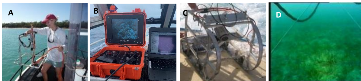
Figure 6. (A-B) Shallow subtidal assessments of seagrass meadows using digital camera mounted on a 0.25m 2 drop frame, and (C-D) offshore underwater sled tows with digital camera.
