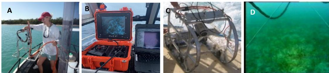
**Figure 6.** (A-B) Shallow subtidal assessments of seagrass meadows using digital camera mounted on a 0.25m<sup>2</sup> drop frame, and (C-D) offshore underwater sled tows with digital camera.
