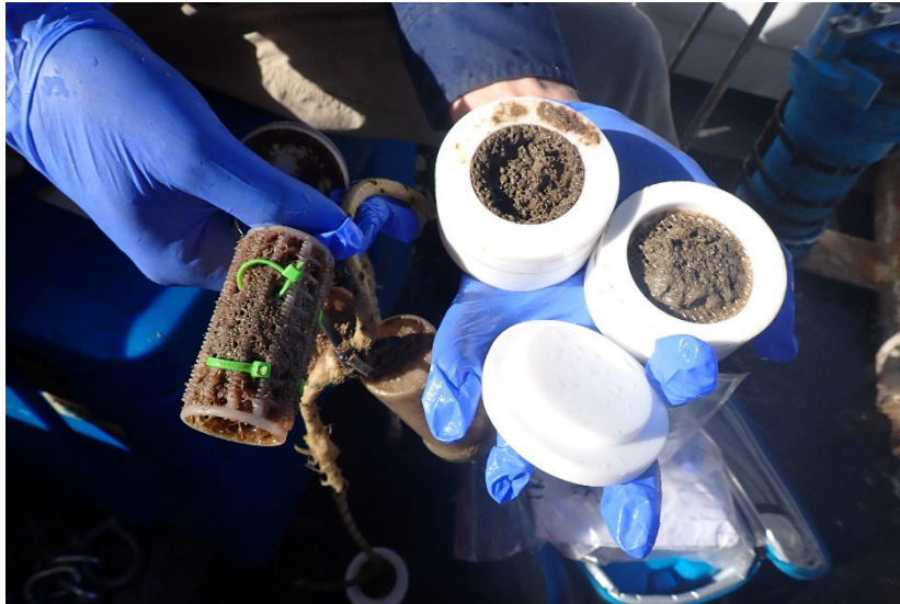
Figure 2-2. Pesticide monitoring passive samplers retrieved from Euri Creek (AP_AMB1) in December 2020. Note: biological growth on the samplers.
