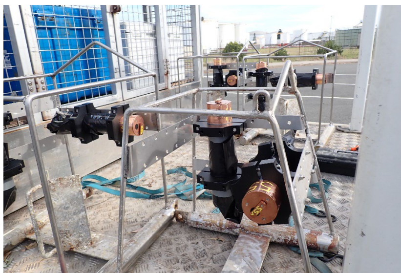
Figure 2-3. Water quality loggers attached to instrument frames ready for deployment to the seabed. The horizontally orientated logger is an NTU-LPT turbidity logger, and the vertically orientated logger is a MS9-LPT multispectral light logger manufactured by Insitu Marine Optics.
