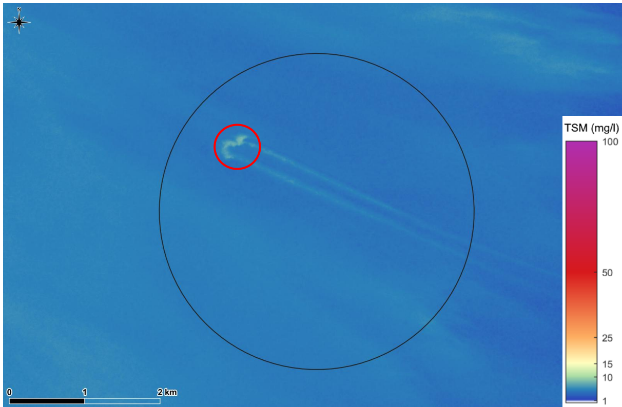
Figure 63. Satellite-derived TSM of DMPA on 11/08/2026. The red ellipse shows a local plume from a recent placement (0.5 hours prior) by the TSHD Brisbane.
