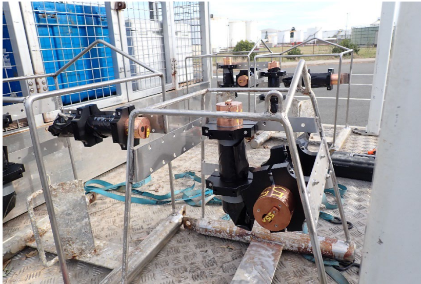
Figure 2-2. Water quality loggers attached to instrument frames ready for deployment to the seabed. The horizontally orientated logger is an NTU-LPT turbidity logger, and the vertically orientated logger is a MS9-LPT multispectral light logger manufactured by Insitu Marine Optics.
