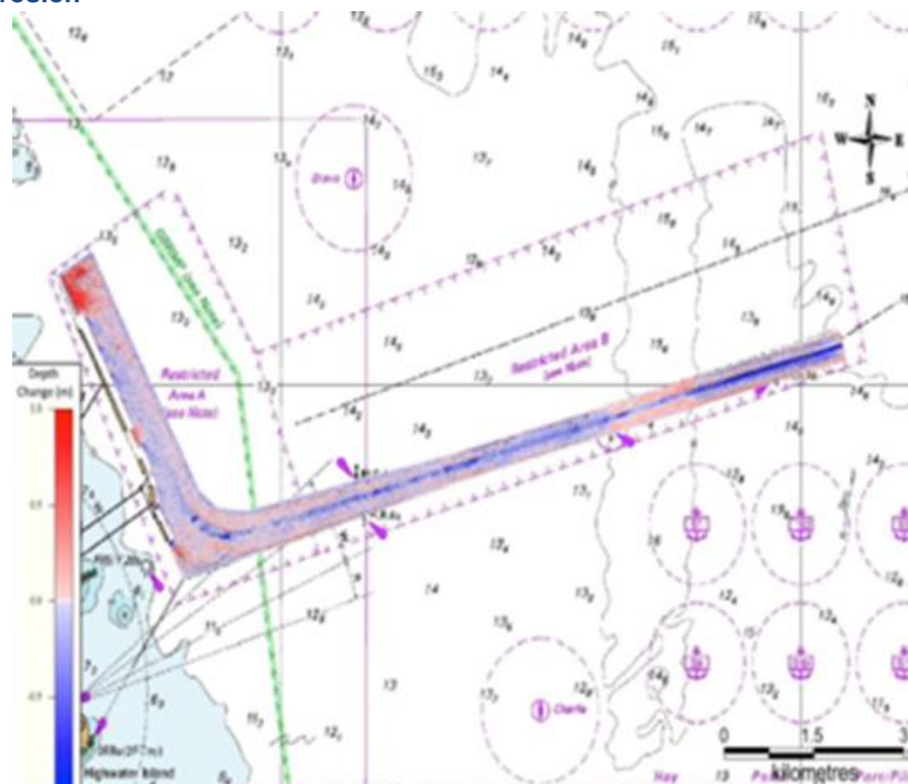
Figure 8: Difference in bathymetry (February 2007 to October 2015) red represents areas of accretion and blue areas of erosion
