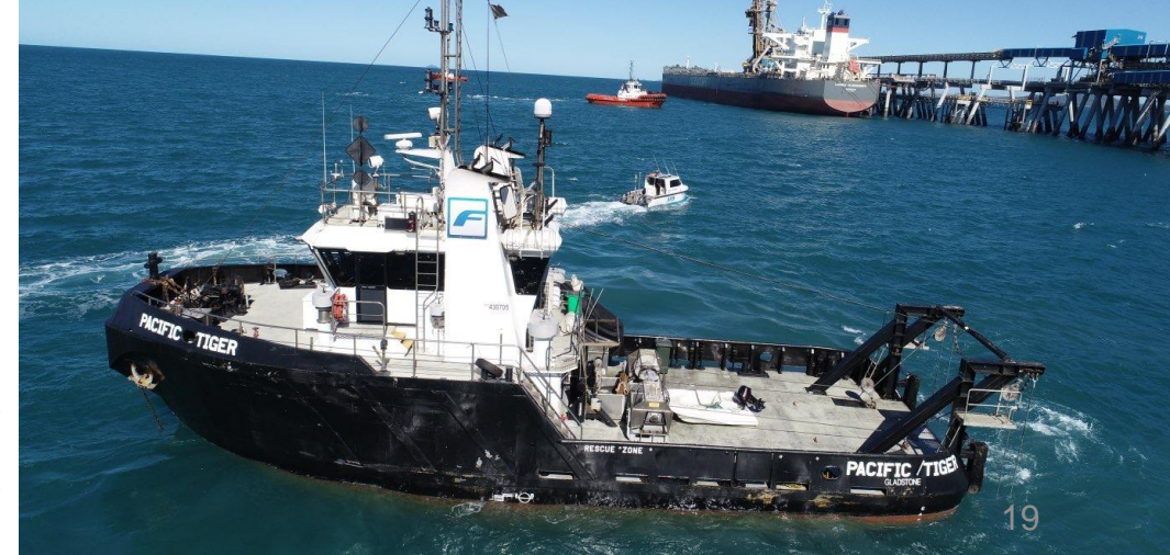
(Above right and below) Image of bed levelling progress at Half Tide Tug Harbour from 2021 campaign, and Pacific Tiger, the bed-levelling vessel, at the Port of Hay Point in 2021.
