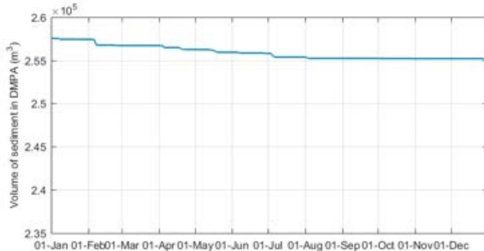
Figure 63. Time series showing the change in volume of placed sediment in the Mackay DMPA over 12 months.
