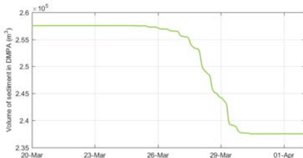
Figure 64. Time series showing the change in volume of placed sediment in the Mackay DMPA over a TC.
